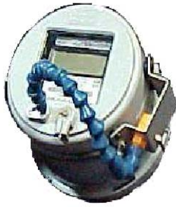
Connect Meter Pickup (Labeled "External")
