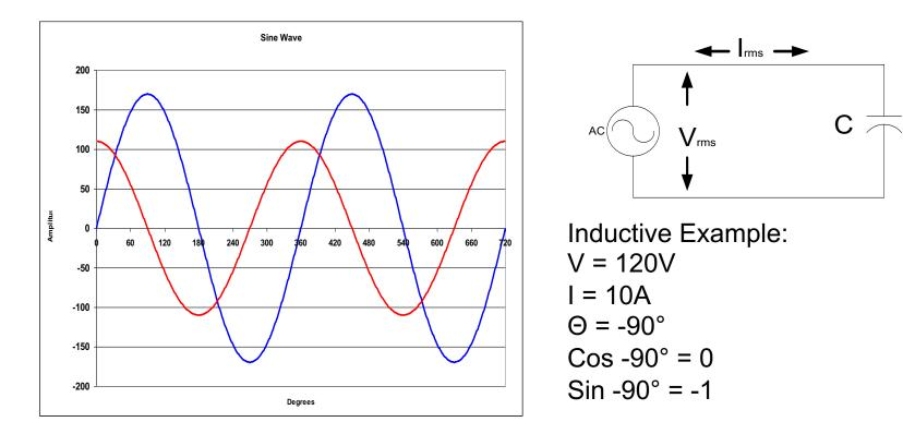
Active Power (W) = V I cos ( $\theta$ ) = 120 \* 10 \* 0 = 0 W Reactive Power (VAR) = V I sin ( $\theta$ ) = 120 \* 10 \* -1 = -1200 VAR Apparent Power (VA) = V I = 120 \* 10 = 1200 VA
