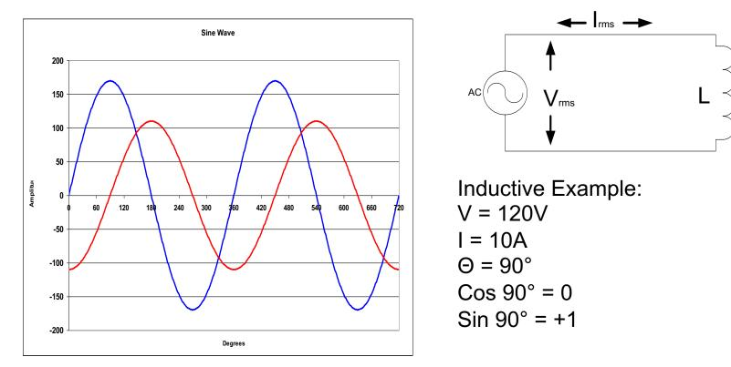
Active Power (W) = V I cos ( $\theta$ ) = 120 \* 10 \* 0 = 0 W Reactive Power (VAR) = V I sin ( $\theta$ ) = 120 \* 10 \* +1 = +1200 VAR Apparent Power (VA) = V I = 120 \* 10 = 1200 VA
