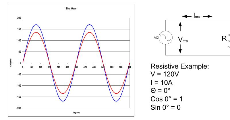
Active Power (W) = V I cos ( $\theta$ ) = 120 \* 10 \* 1 = 1200 W Reactive Power (VAR) = V I sin ( $\theta$ ) = 120 \* 10 \* 0 = 0 VAR Apparent Power (VA) = V I = 120 \* 10 = 1200 VA
