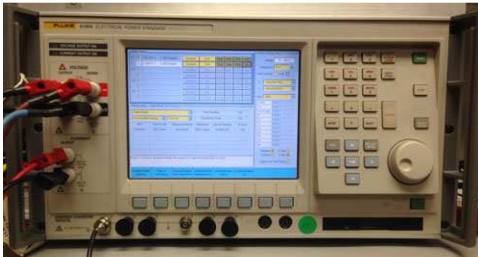
Fluke 6105 Front Panel With Connections
