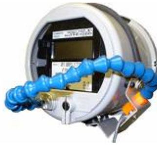
Hook up pulse pickup to meter
